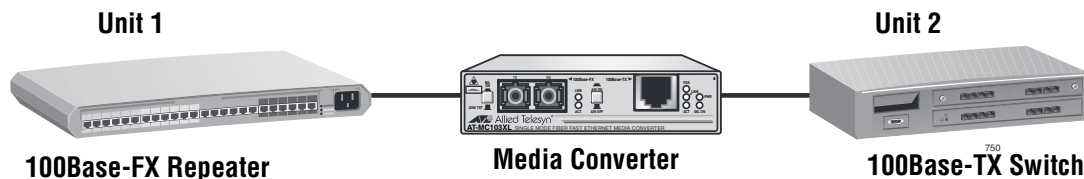
Figure 8. Example of a Duplex Mode Mismatch
